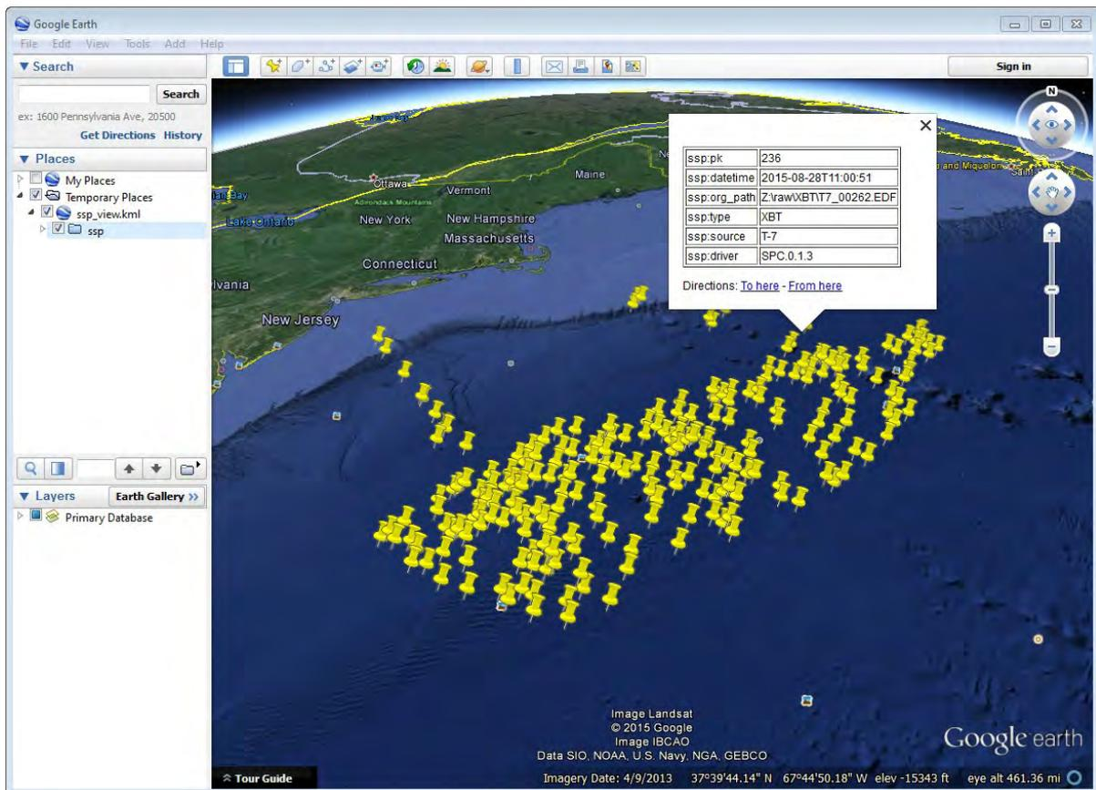
**Figure 6 :** Loading result of the exported metadata, using KML, in Google Earth
