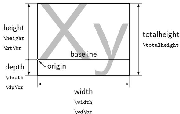
Figure 1: Box dimensions. Shown are also the  $\text{\LaTeX}$  macros and the  $\text{\TeX}$  primitives. Here  $\backslash\text{br}$  stands for a box register. Note that the depth is a positive values on its own downwards pointed axes.
