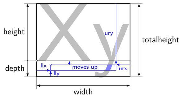
Figure 4: Trimming with  $ury > height$ . In this case the resulting box falls down to the original baseline
