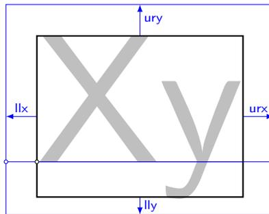
Figure 7: Marginbox. The  $llx$  and  $urx$  are added to the left and right and increase the width. The  $ury$  is added to the height and  $lly$  to the depth of the box. This keeps the baseline at the original position.
